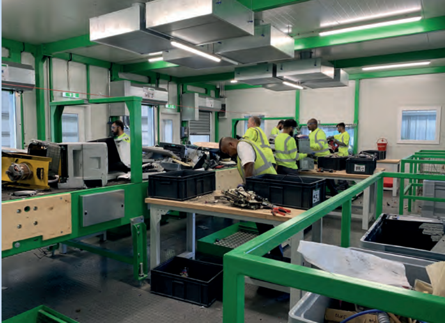
At the first stage, contaminants such as batteries, capacitors, cables, toner cartridges, display screens, circuit boards or solid parts are dismantled and processed during manual pre-sorting.
