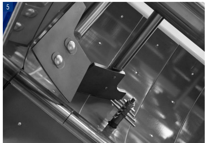
4d Mixing tools in chilled chrome cast iron design
