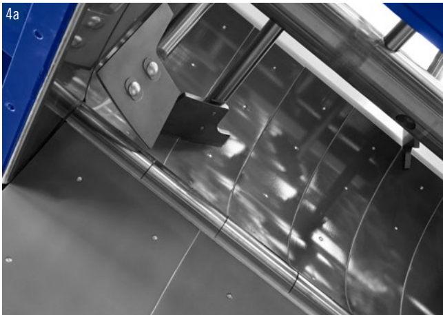
4a Smooth mixing tool with steel blades for materials with a density of <1.4 \text{ t/m}^3 .
