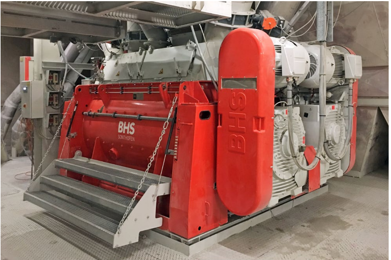
Dry Powder Batch Mixer DMX 4900 with hinged maintenance platforms.
